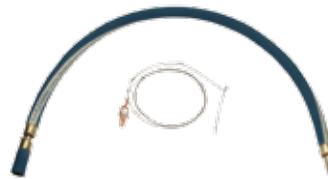
Static Protection Kit - includes 4 ft. synthetic rubber cross-linked poly- ethylene grounded hose with brass fittings with 3/4" MNPT, ground wire, and clamps - P/N 107429
